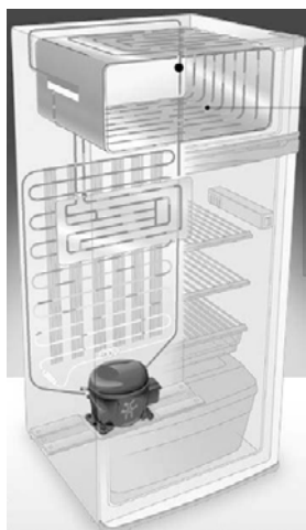
Figure 9-7: Household refrigerator (picture courtesy of Embraco, visit http://www.embraco.com/ingles/lancamentos.htm to see an animation of the refrigeration circuit).
